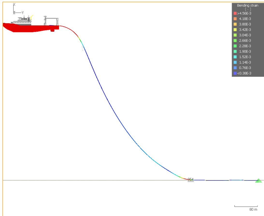
Model View - Critical Plastic Strain Location - Payout Complete
