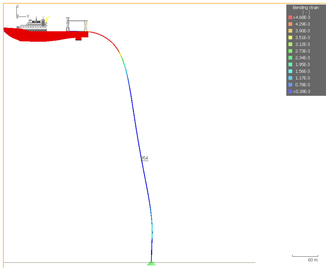
Model View - Critical Plastic Strain Location - Payout at 1628s
