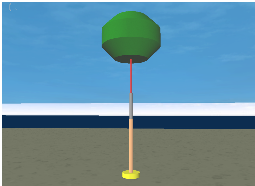
Flexcom model of Submerged Point Absorber
